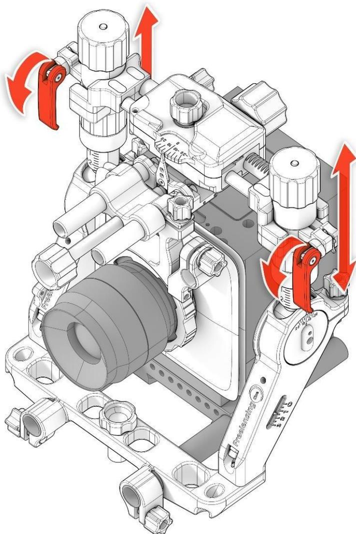
ADJUSTING SCREW (M3) from the locking cam for Y-shift (pay Special attention to the pressure of this screw, as it could loosen due to vibrations during transport).
