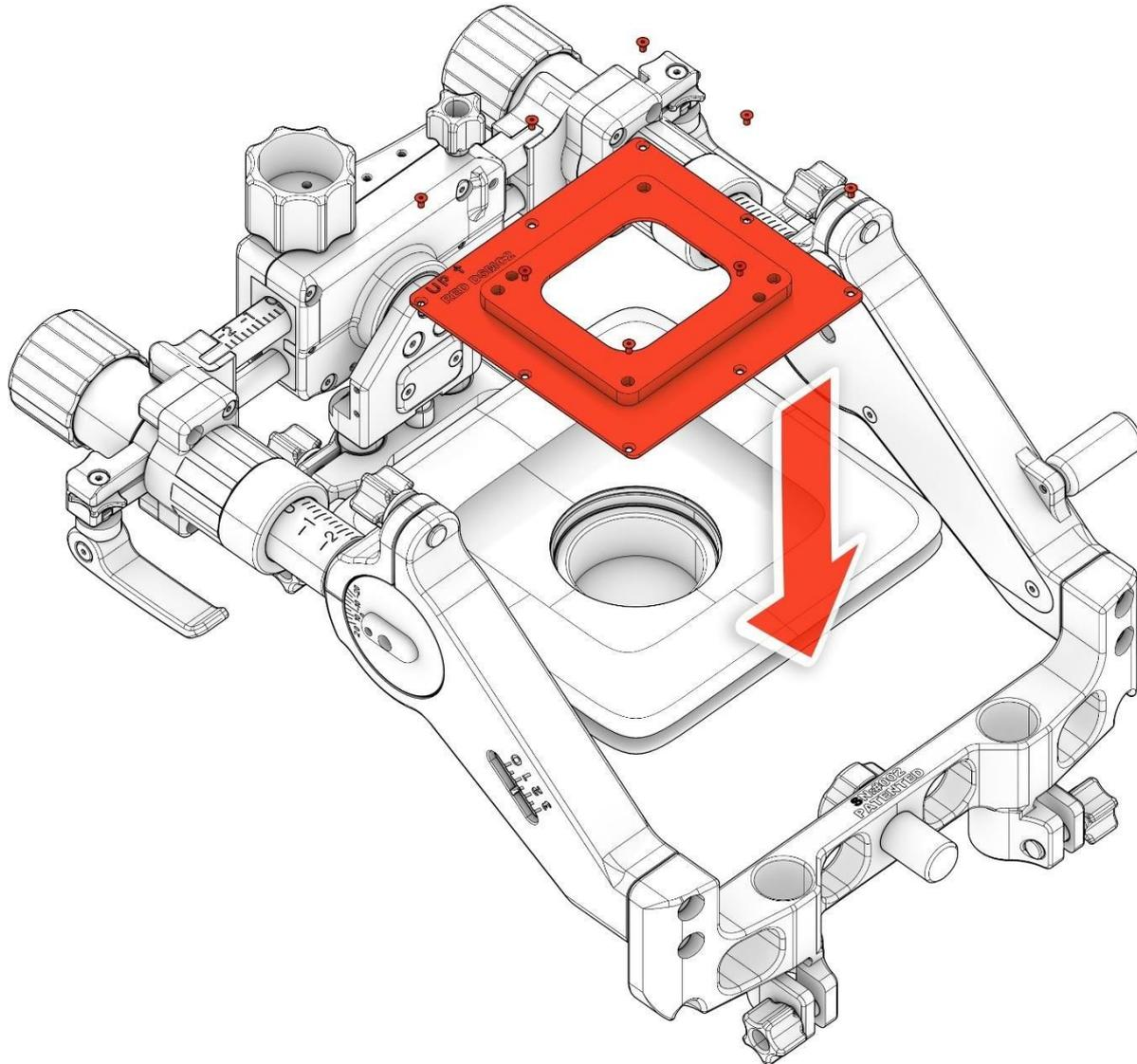
For SONY VENICE & RED DSMC2, when attaching the screws, the operator must always look at the "UP" side of the mount → and see the position of the upward arrow.
