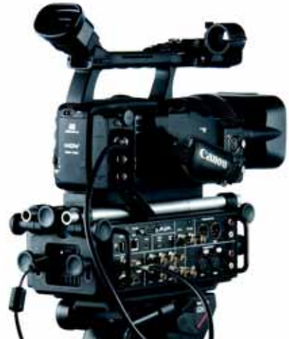
Ki Pro with Exo-skeleton and optional endplates with user-supplied accessory rods.
